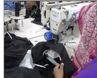
Photo of non-conformity Finding 7.17 Eye Guard displaced.JPG
